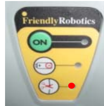
Figure 1 Wire disconnected indicator is blinking
